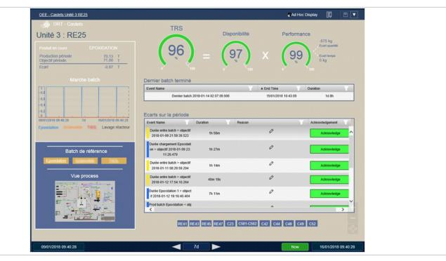
DRT's management utilizes PI Vision dashboards to track Overall Equipment Efficiency (OEE) metrics and continuously improve productivity and efficiency at the plants.
