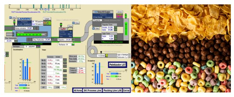
Using the PI System's Asset Framework, the Valls plant has created a digital twin of plant operations and increased OEE from 67% to 80%.
