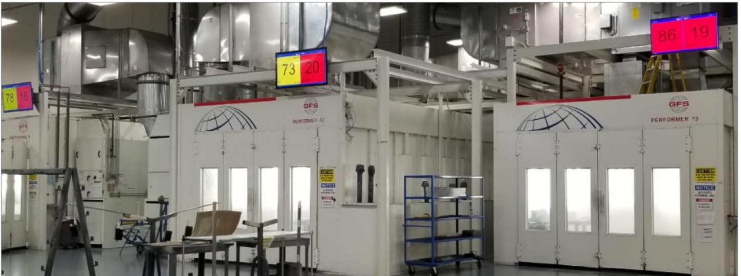
PI Vision displays with color-coded alarms help to monitor temperature and humidity in real time inside the paint booths for drones.
