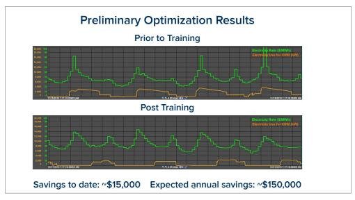
By visualizing chiller operation alongside fluctuations in energy rates, building operators at UC Davis are able to time energy usage more efficiently.
