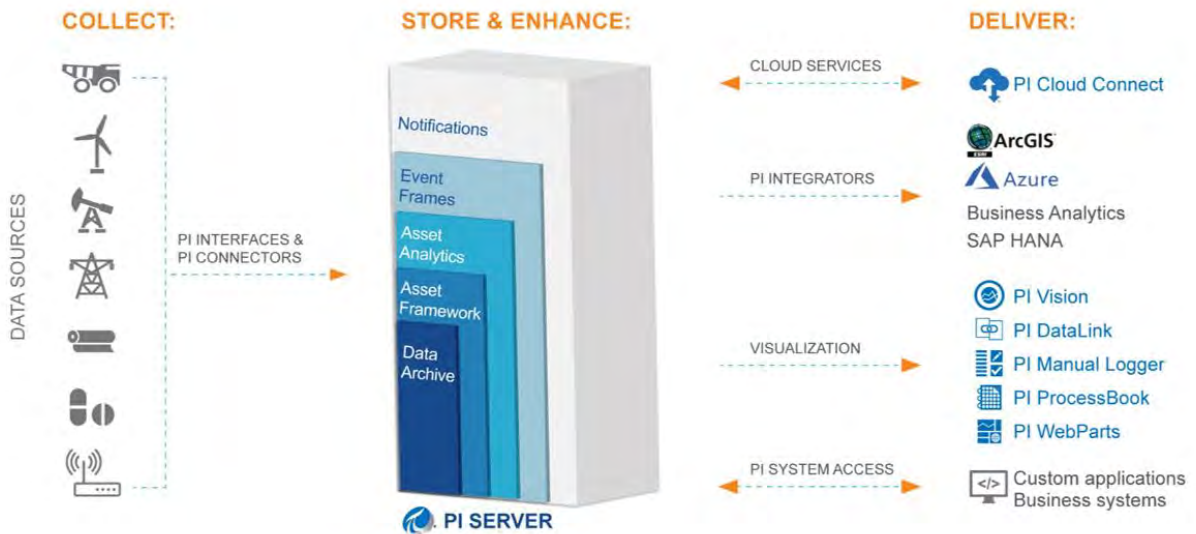
Figure 2-1. OSIsoft’s PI System Modules and Processes
